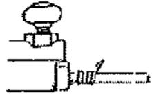
1. Select the hole that best fits the size wire being used. Wrap the wire around the rod as pictured.
