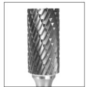
**DOUBLE CUT**Basically a standard cut tool, with cuts made on the left hand spiral. The design produces a finer finish on material and reduces the size of the chips and slivers. It gives greater tool control.
